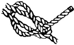
**Sheet Bend** Also known as a Weaver's Knot and is used aboard ships for joining small or medium sized ropes. Popular also in textile mills for joining threads or yarn.
